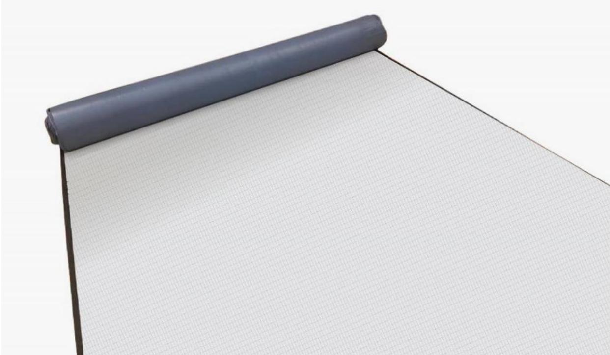
CANVAP S is a self-adhering vapor barrier membrane used in insulated roofing and wall systems, composed of a tri-laminated woven polyethylene film on the top surface, a silicone release film on the bottom surface, and a polymer-based adhesive that allows installation in cold climate without primer.
